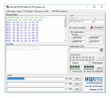
Debugging and testing tool for products with a serial port (PortBox, I/O Controller, IP Relay, PortStore).
