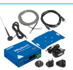
Ares 12 set Bulk + temperature sensor, power adapter, GSM antenna, USB cable and CD with software
