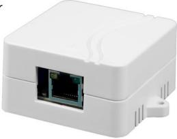
RS-485 protocol is compatible with Temp-485 sensor, measured values of temperature and humidity are read over RS-485 bus as two independent measurements, each with different address. So each H-Temp device has two different RS-485 communication addresses. Capital letter stands for temperature address, small letter for humidity address.
