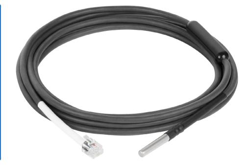
If you need reliable temperature sensor for industrial applications, the Temp-1Wire Pt100 is the right choice. Temperature sensor based on high precision Pt100 probe offers high accuracy over a wide temperature range, IP67 protection and 8-point calibration. The sensor is powered from the RJ11 port, connect it directly to the 1Wire sensor port of HWg device.
