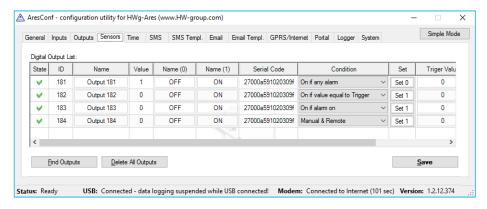
It is possible to connect the External Outputs module\* via the 1-Wire UNI interface to the Ares 12 device. This module provides 4 NO/NC relay outputs with maximum load up to 1A/30VDC or up to 0.5A/50VAC.
