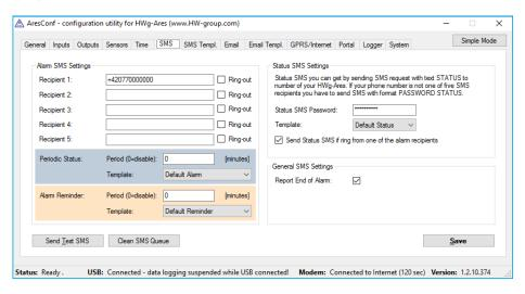
Use this tab to configure alarm text message (SMS) recipients. Each recipient phone number is also authorized to request information from Ares by dialing the unit's phone number and to send SMS commands without a password.
