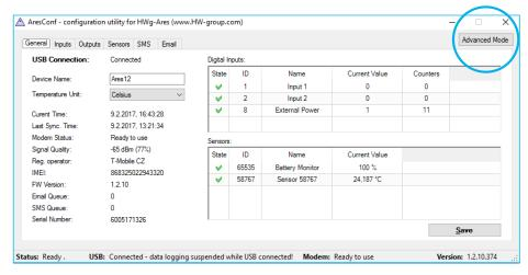
2 In AresConf, first switch to Advanced mode by clicking the button in the top right corner of the window, then go to Portal tab.
