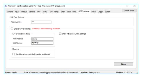
Use this tab to configure the GSM and internet connection details.
