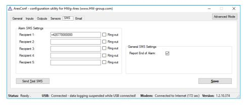
Use this tab to configure alarm text message (SMS) recipients. Each recipient phone number is also authorized to request information from Ares 12 by dialing the unit's phone number and to send SMS commands without a password (see *Advanced settings*).
