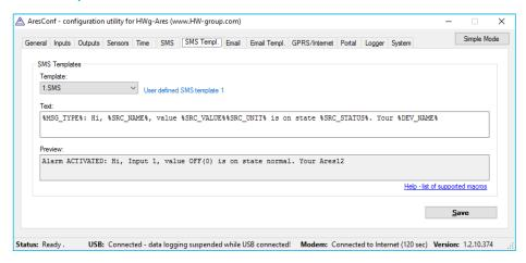
Use this tab to define the formats of individual messages, e.g. to distinguish temperature alarm messages from humidity alarm messages or to define the contents of status and reminder messages.
