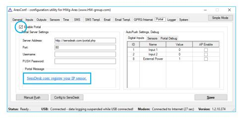
Tick the Enable Portal option and save the changes using the Save button in the bottom right corner of the window. Then click the Manual Push button in order to activate the portal function. Instead of "Portal disabled", a link SensDesk.com: register your IP sensor should appear in the Portal Message field. Click this link in order to get to the SensDesk portal.
