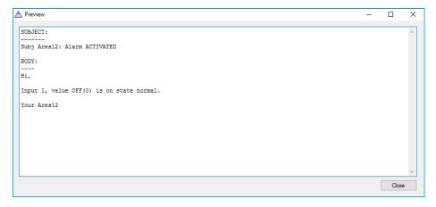
Use this tab to define the format of individual messages, e.g. to distinguish temperature alarm messages from humidity alarm messages or to define the contents of status and reminder messages.
