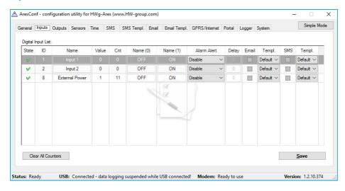
Use this tab to configure basic and advanced properties of digital inputs:
