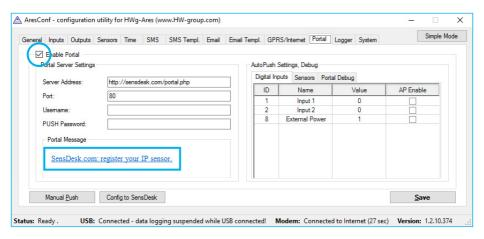
Tick the Enable Portal option and save the changes using the Save button in the bottom right corner of the window. Then click the Manual Push button in order to activate the portal function. Instead of "Portal disabled", a link SensDesk.com: register your IP sensor should appear in the Portal Message field. Click this link in order to get to the SensDesk.com portal.
