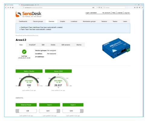
By activating the account, you will be redirected to the Devices > View page. At this moment, the data-sending period is set to 10 seconds to show the sensors functionality. This page is active only for approximately 15 minutes after the activation, then the logging period changes to 15 minutes.
