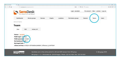
If you check Teams link, you will find your PUSH password. This password, together with your login name, identifies the device in communication with your account and in communication of mobile applications with SensDesk. The password cannot be changed and for a security reason it is different to the login password.
