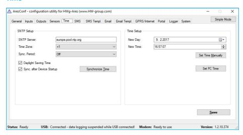
Use this tab to configure the current system time. The time can be set either manually in *Time Setup*, or automatically over the internet.
