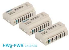
Measures power consumption using external M-Bus meters.
