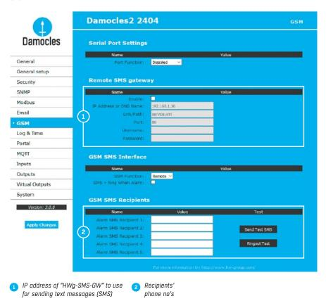
**Note:** We recommend to use HWg-SMS-GW3 for sending text messages. One central SMS gateway for all HW group devices in a single LAN.
