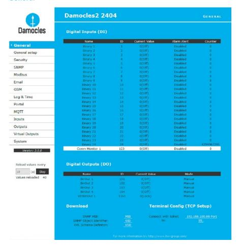
The main page with the overview of DI and DO states automatically reloads at configurable intervals (by default every 10 seconds, can be changed easily).
