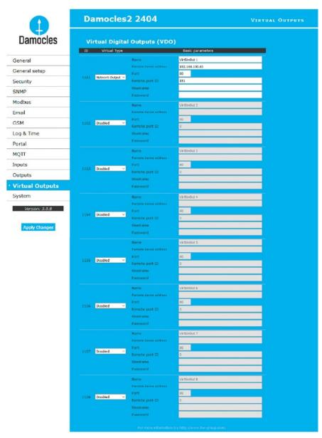
Virtual Outputs allow the use of outputs of other Poseidon2 or Damocles2 units (Box2Box). The communication uses the TCP protocol and updates take place every 60s. For more information, see Web interface - Virtual Outputs.
