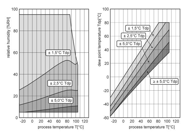
Accuracy of computed absolute humidity for compressed air measurement up to 25 bars.
