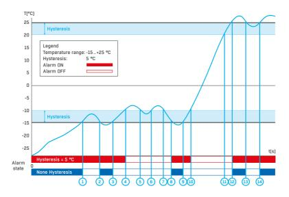
Within the internal 5°C hysteresis band, the alarm would be activated in **point 8** and would end in **point 9**. Because of the hysteresis function, the alarm is extended until the temperature reaches the end of the hysteresis zone (point 10) 5 °C + (-15 °C) = -10 °C.
