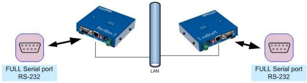
Extension of the serial port over TCP/IP. The serial port is set to 19,200 Bd, 8N1, SW handshake,
