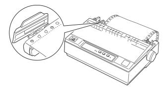
5. To separate the incoming paper from the printed paper, attach the paper guide by holding it horizontally and fitting its notches over the printer's mounting posts as shown below. Then slide the paper guide toward the front of the printer until you feel it click.
