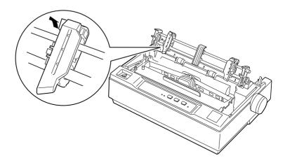
5. Insert the paper into the paper slot as shown below and pull it up. Position the paper using the scale on the printer as a guide. The printer prints to the right of the position marked 0.
