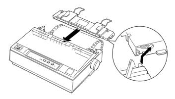
6. Slide the left edge guide to the center until it stops at the guide mark. Then slide the right edge guide to the opposite guide mark
