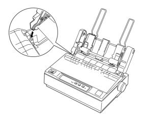
5. Slide the left paper guide so it is aligned with the triangle mark. Next, slide the right paper guide to roughly match the width of your paper. Slide the paper support midway between the paper guides.
