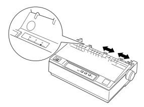
4. Make sure your paper has a clean, straight leading edge. Open the sprocket covers. Fit the first holes of the paper over the sprocket pins and then close the sprocket covers. Slide the right sprocket unit to remove any slack in the paper and lock it in place. Now the paper is in the paper-park position.
