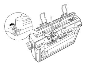
2. Guide the interface cable through the slot on the side of the printer so that it does not block the paper supply as shown in the illustration on page 1-16.
