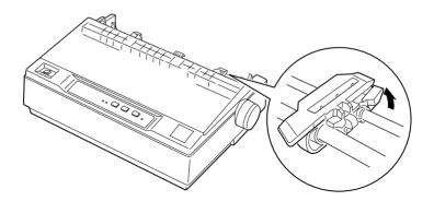
3. Slide the left sprocket unit using the scale on the printer as a guide. The printer prints to the right of the position marked 0. Push the sprocket lock lever back to lock it in place. Then slide the right sprocket unit to match the width of your paper, but do not lock it. Move the paper support so it is midway between the sprocket units.
