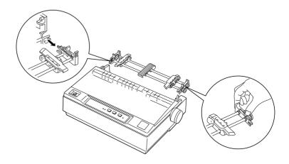
3. Lift the tractor forward to the mounting slot at the top of the printer and tilt it into place as shown below. When you push the tractor onto the posts, you should feel the notches snap into place.
