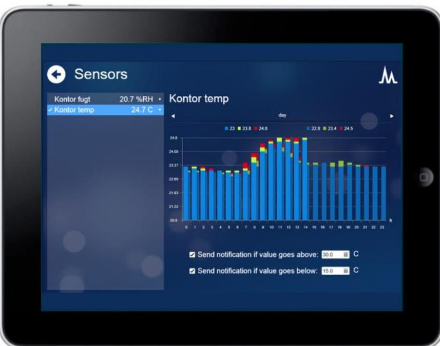
can be set in order to activate an email and/or SMS text notification when defined upper and a lower limits are reached. The defined limits work independently of settings made in the device itself. An alarm situation turns the sensor name red. [Menu: Leaks](#)
